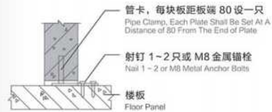
③ 板长 > 4米 | 管卡法 (钢板可在任一方向固定) Board Length > 4 m | Pipe Clamping (Steel Plates Can Be Fixed in Either Direction)
