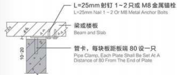
① 管卡法 (钢板可在任一方向固定) Pipe Clamping (Steel Plates Can Be Fixed In Either Direction)
